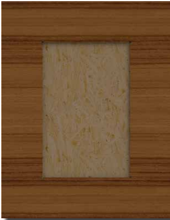
wood panel with prepared pocket milling
