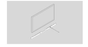
Mark the screw locations and remove the wall mount bracket for now.
